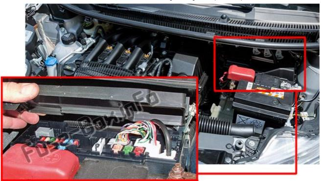
Unclip the cover, pressing on the right on lug E, to gain access to the fuses.
