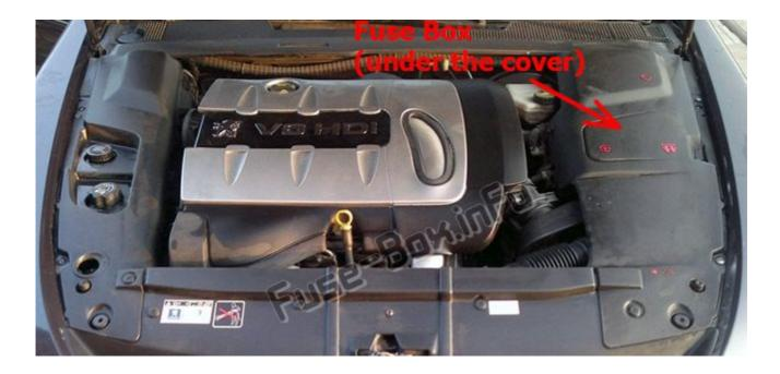
To access the fuses located in the engine compartment, remove the cover and unclip the fusebox lid.
